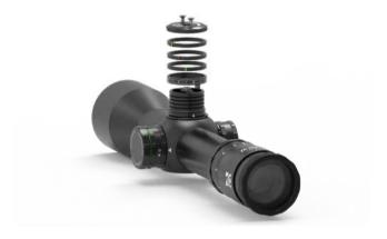
Lifting the rotating cap unlocks the turret and the height can be adjusted by clicking. Once you have set the elevation adjustment to the first distance required, press the rotating cap down again to lock the turret.
