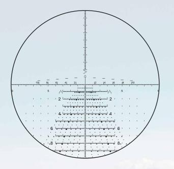
Horus Grid: The uniform 0.2 milliradians Horus Grid allows you to easily compensate for bullet drop for any ballistics and density altitude. The solid grid provides numerous precise aiming points for extreme precision, not requiring the user to hold out in space. Additionally, the grid provides fast and accurate Second Shot Corrections.
