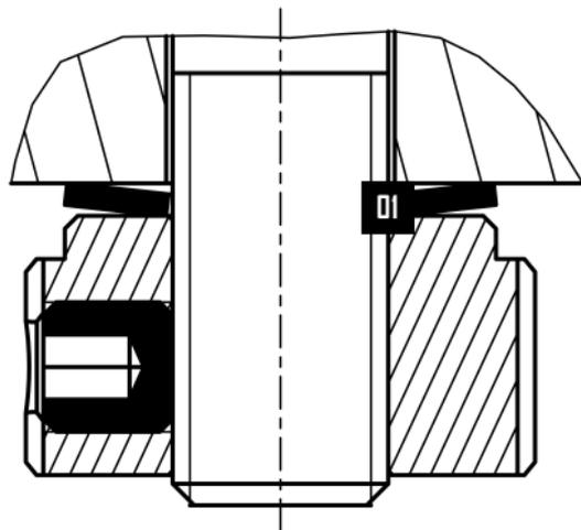
01 Small diameter of the conical spring washer need to be in contact with the knurled adjustment nut
