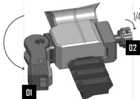
01 Unlock and open the tension lever
