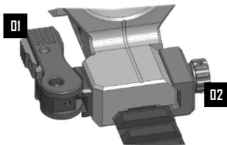
01 Lever in tensioned and locked position
