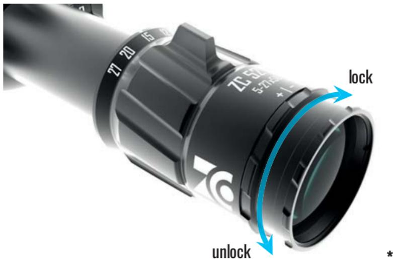
4. While looking through the scope at an all-white background, with a moderately fast speed, turn the diopter adjustment until the reticle goes out of focus. The speed of turning should be fast enough that your eye isn't able to compensate to focus the reticle.
